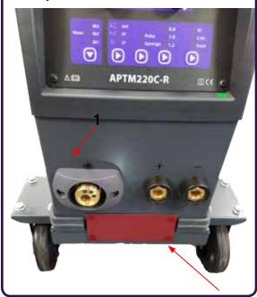
STEP 4 - Fix the rear bracket to the trolley using 2 new screws
