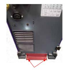
STEP 5 - Fix the top bracket between the trolley and the machine using 2 new screws and 2 existing in the top of the machine
