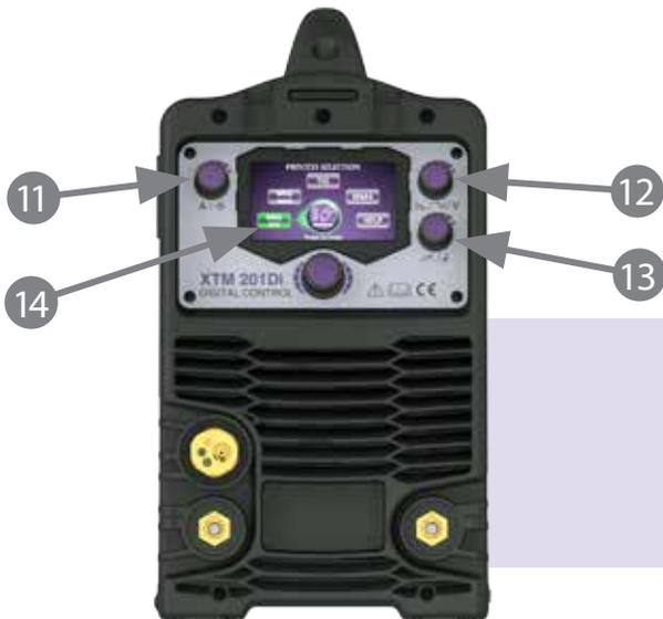
11. Amperage / Wire Speed Adjustment
