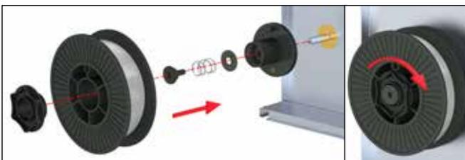
**Note: There is a friction brake on the reel hub assembly to prevent the wire spool over running when welding stops; ensure this is slackened to the minimum setting. It can be adjusted by means of the nut visible when the plastic hand nut is removed.**
