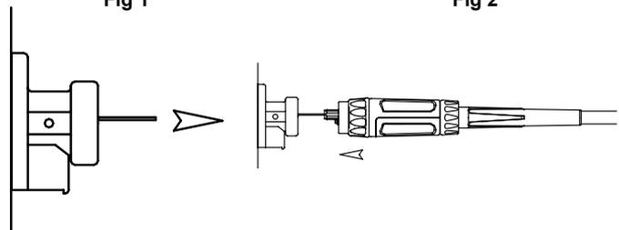
**Note: To aid the initial location of a new torch and to prevent damage to the gas nipple O-Ring a very light application of grease to the O-Ring is beneficial.**
