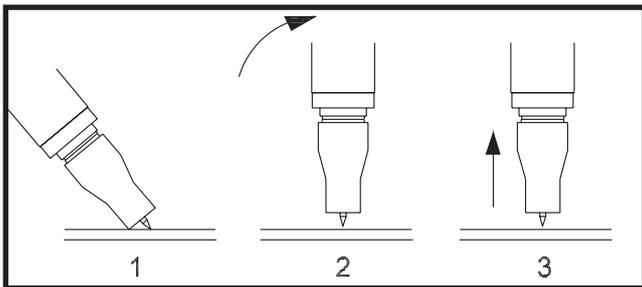
At the end of the weld release the trigger and allow the power and gas to switch off before moving the torch from the weld.
