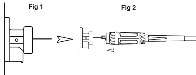
**Note: To aid the initial location of a new torch and to prevent damage to the gas nipple O-Ring a very light application of grease to the O-Ring is beneficial.**
