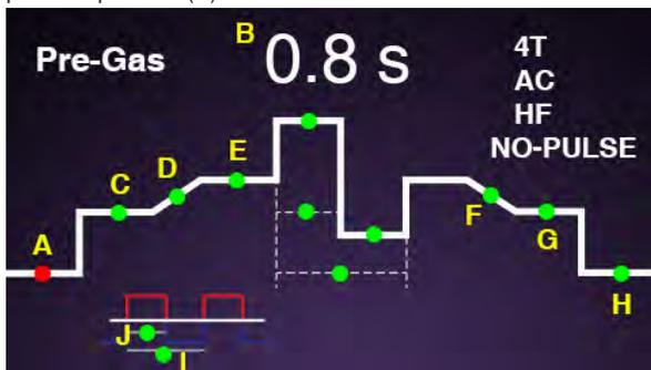
9) Press the control knob to select the parameter. The red LED will now flash. Adjust the value by rotating the control knob. This can be adjusted from 0.1 to 0.3 seconds. The value is displayed on the digital display (B) Press the control knob again to accept the setting.
