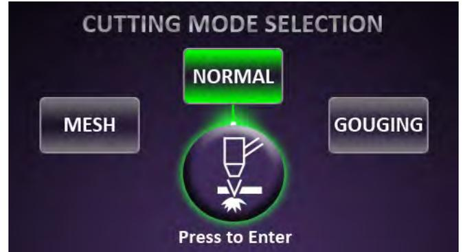
Select the material type to be Cut or Gouged
