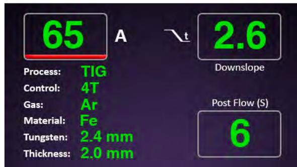
Adjust downslope and post flow to user preference using the knobs on the right of the screen.
