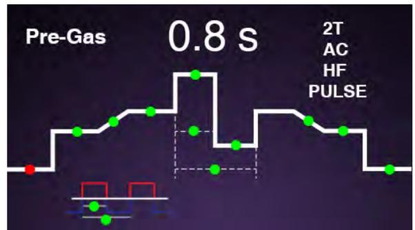
To Select and adjust Pre-Gas, Slope Up, Welding Current, Slope Down, or Post Gas do the following:
