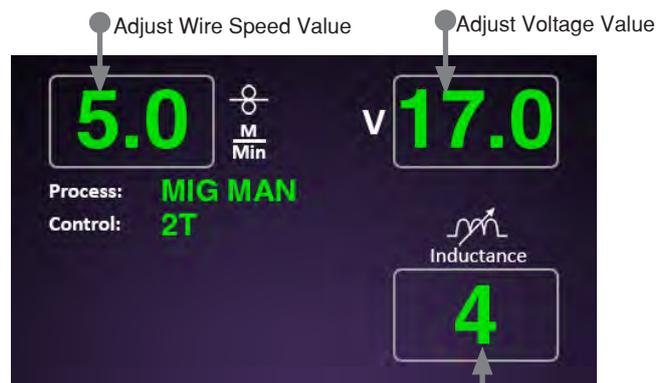
In manual mode you can adjust the parameters using the controls indicated.
