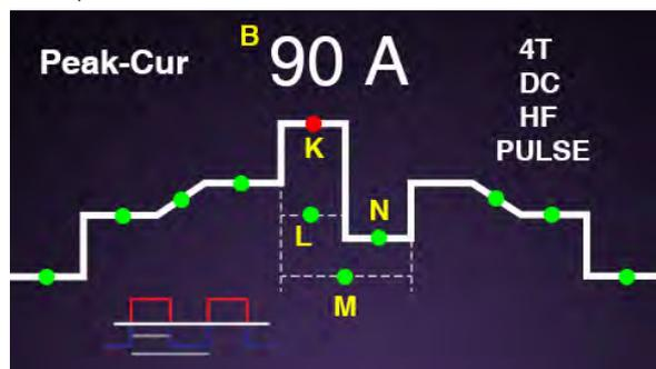
4) Rotate the control knob to move the LED to the Peak duration (L) This can be adjusted from 5 to 100% Peak duration is the percentage of time the peak current is on relative to the background current. 30% is a good starting point.
